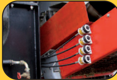
Quarrying – Greasomatics fitted remotely 5 metres away from the conveyor bearings
