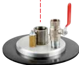
P/N OE11/34 Follower plate ø 310 mm with NBR seal ring and suction tube adaptor ø 45 mm (for drum with internal ø from 260 to 310 mm).
