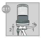
For EP/CONNECT: Move the connector outwards by unscrewing the F1/4 fitting. Connect the power plug.
