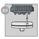
Insert the pin of the module in the notch of the base.
