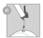
Prime lube point and remove nipple.
