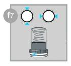
Cartridge empty/ unprimed pump: alternating blue lights for 1s, every 10s, during 4h after expulsion.
