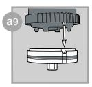
Insert the pin of the module in the notch of the base.
