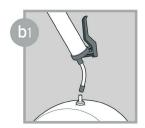
Prime lube point and remove nipple.
