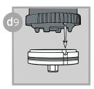
Insert the pin of the module into the notch of the base.
