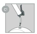
Prime lube point and remove nipple.
