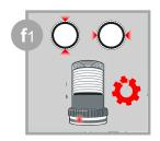
Alternating red light for 1s, every 10s: Gearbox broken or blocked. VISIO stops after 3 trials.
